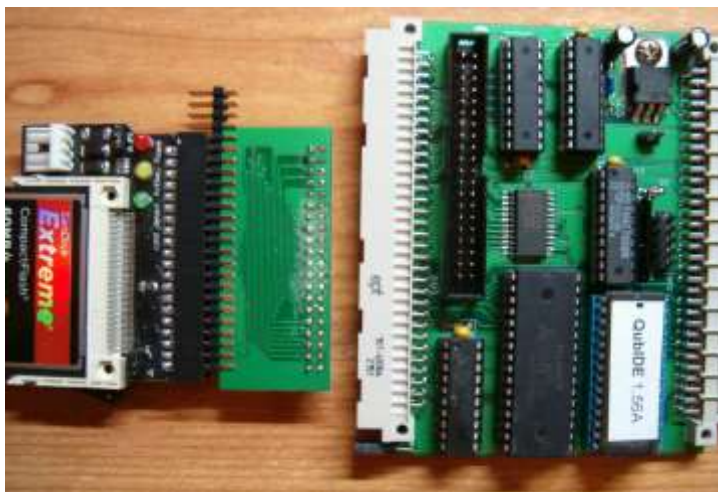
Picture of the new Qubide with through connector (right) and right angle adaptor board (centre) for the Compact Flash adaptor card (left)
